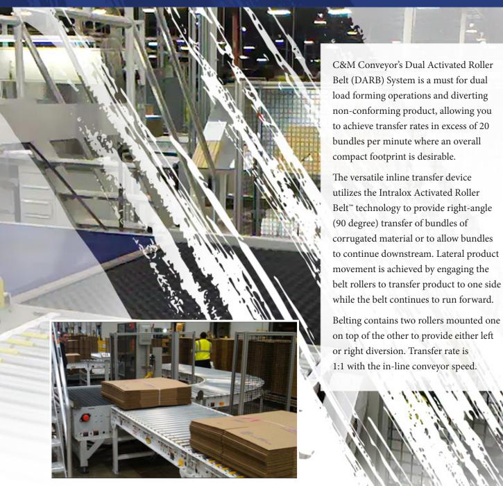
*C&M* is the exclusive licensee for Intralox Activated Roller Belt for North and South America for the corrugated and folding carton market. Units shown incorporate licensed technology which is patented.
